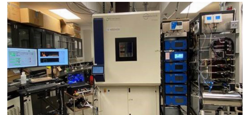
The AQ-SPEC Sensor Environmental Test Chamber (SEnTeC-2) will be used with the ASTM test standards work.
