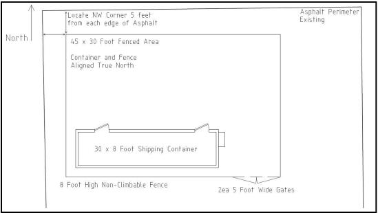
Figure 3 LAX - 2 Monitoring Site Detail
