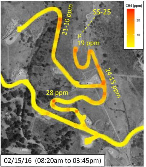
• Elevated methane concentrations (in the 10 to 24 ppm range) were measured near/around the SS-25 well, probably from multiple naturally occurring holes on the side of the hill; increased methane levels (up to 19 ppm) were also measured ~80 ft S of the SS-25 well's head
