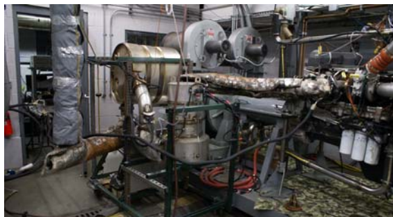
Figure 10: Volvo MD11 engine with ADECS on the test bed in WVU Engine and Emissions Research Laboratory (EERL)
