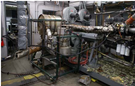
Figure 1: Volvo MD11 Engine with ADECS on the Test Bed in WVU Engine and Emissions Research Laboratory (EERL)
