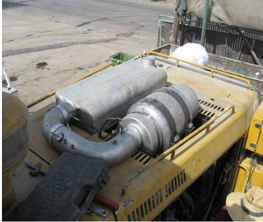
Figure 1. DPF and SCR Catalyst on Loader
