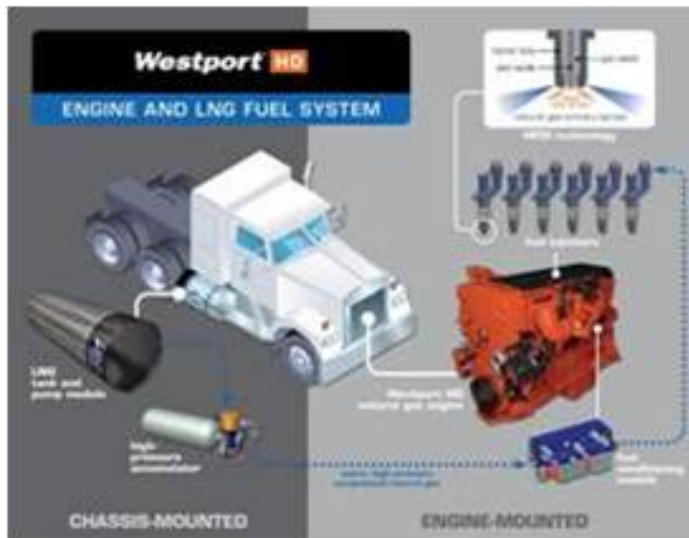
Figure 14: Westport Engine and LNG System
