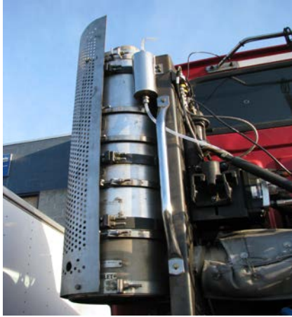
Figure 2. SCRT system installed on the test vehicle.
