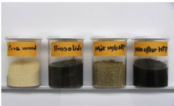
Figure 2. From left to right, Biomass, Biosolid, Mixture of biomass and biosolid, Formation of pumpable mixture of biomass and biosolid after the hydrothermal pretreatment (43% solid loading).
