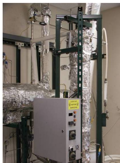
Figure 17: Bench Scale SHR-WGS System
