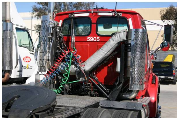
Figure 15: Truck Equipped with SCRT™
