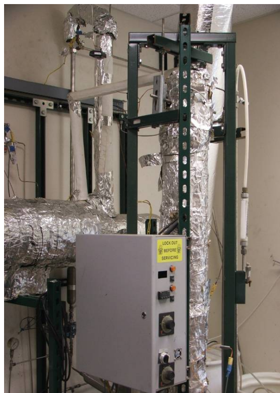
Figure 1. Picture of SHR-WGS systems. SHR (left) was modified and new WGS (right) was added.
