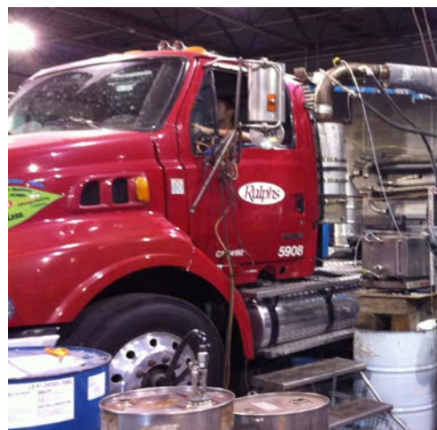
Figure 1. Test Vehicle during chassis dynamometer testing.
