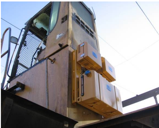
Figure 2. DPF/SCR Components on Excavator
