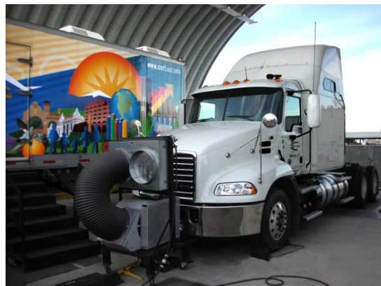
Figure 1: Truck being tested on chassis dynamometer
