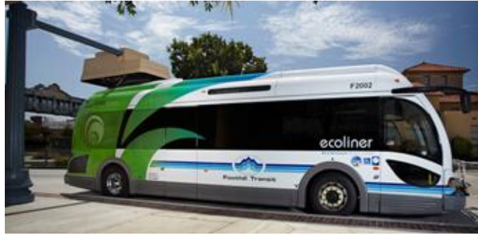
Figure 14: Foothill Transit's Electric Bus Charging in Pomona
