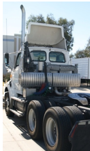
Figure 2: SCCRT Typical System Installation
