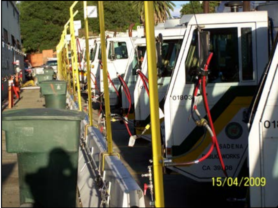
Figure 2: City CNG Refuse Trucks at Slow-fill Filling Posts
