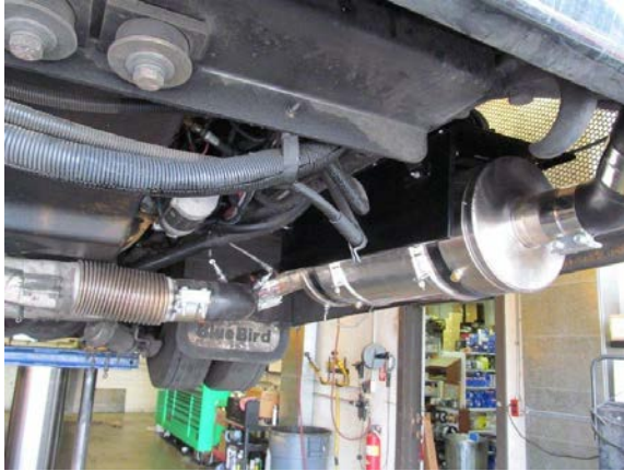
Figure 1: ESW Thermacat installed on Bus 62
