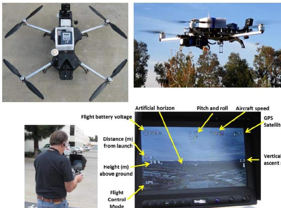
Figure 4 Commercially available multi-rotor UAV (i.e. quadcopter) outfitted with a UV photometric (Federal Equivalent Method; FEM) ozone analyzer. This unit is equipped with precise flight controls with first person view, display of flight parameters and air to ground telemetry of key data ( courtesy of T&B Systems; Valencia, CA )
