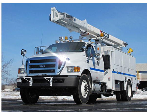
Figure 7: Class 7 Bucket Truck Equipped with Odyne Plug-In Hybrid Drive System
