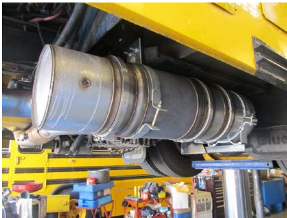
Figure 2: Donaldson LNF installed on Bus 55
