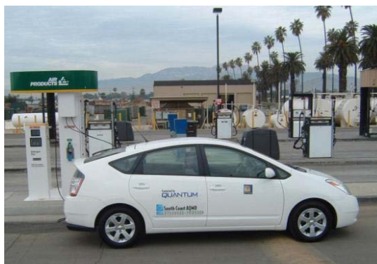
Figure 1: 2008 Toyota Prius Converted to Operate on Hydrogen Fuel
