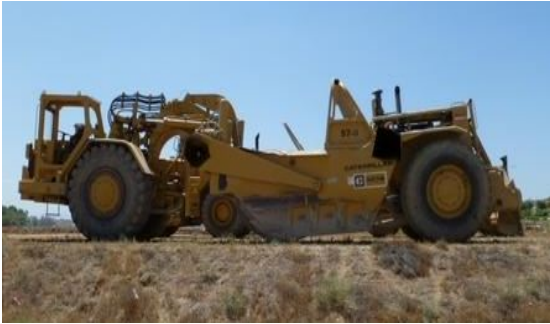
Caterpillar 657B Scraper Repowered to Tier 3
