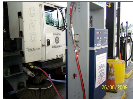
Figure 3: City CNG Street Sweeper at Fast-fill Dispenser
