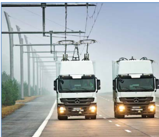
Figure 5: Catenary-Accessible Trucks on the Siemens' Test Track in Berlin, Germany
