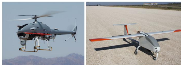
Figure 2 Typical rotary-wing (left) and fixed-wing (right) UAVs used for civilian applications
