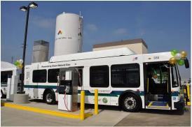
Figure 2: City of Commerce transit bus fueling at the new L/CNG station
