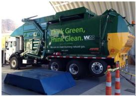
Figure 8: Truck with ISL-G-NZ Ultra Low-NOx Engine
