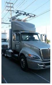
Figure 6: Drayage Truck Connected to Demonstration Catenary System in Carson
