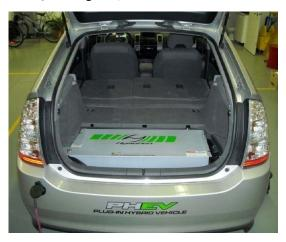
Figure 1: A123 Plug-In Hybrid Conversion
