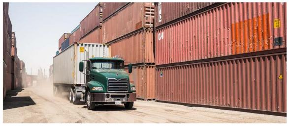
Figure 18: Volvo's PHEV Drayage Truck
