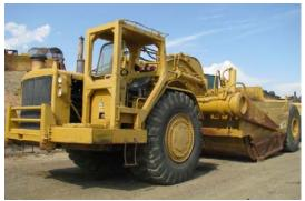
Figure 2: Caterpillar 651B Scraper Repowered to Tier 3
