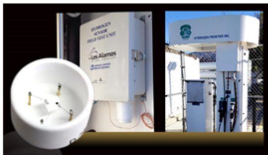
Figure 1: A close-up of a sensor element (left). Hydrogen sensor prototypes were installed at fueling station in Burbank (right) and Chino to assess their performance and long-term stability.
