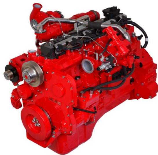
Figure 34: Full Production 2018, 8.9-L Natural Gas Engine Certified at 0.02 g/bhp-hr NO x Emissions
