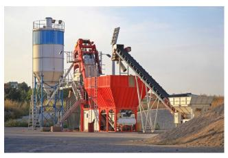
Figure 5f-1: Concrete batch plant
