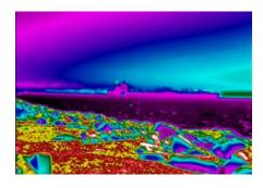
Infrared Cameras: Inspectors can use specialized infrared cameras to view emissions of gases (including methane and VOCs) that would otherwise be invisible to the naked eye. This equipment enables inspectors to scan areas for emissions and quickly check for any large leaks at a facility.
