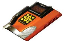
$H_2S$  Analyzers (Jerome Meters): Inspectors can use this handheld instrument to measure hydrogen sulfide gas levels in the air. This information can be used to identify a potential source of rotten egg type odors.
