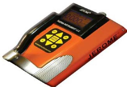
*H<sub>2</sub>S Analyzers (Jerome Meters):* Inspectors can use this handheld instrument to measure hydrogen sulfide gas levels in the air. This information can be used to identify a potential source of rotten egg type odors.
