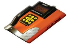
$H_2S$  Analyzers (Jerome Meters): Inspectors can use this handheld instrument to measure hydrogen sulfide gas levels in the air. This information can be used to identify a potential source of rotten egg type odors.
