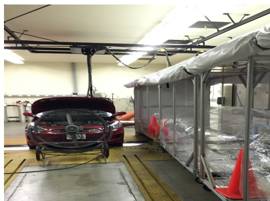
Figure 1: A vehicle is being tested on the chassis dynamometer with the mobile environmental chamber collecting primary emissions.
