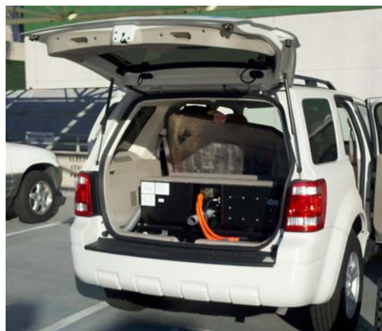
Figure 1: Enerdell battery integrated by Quantum Technologies
