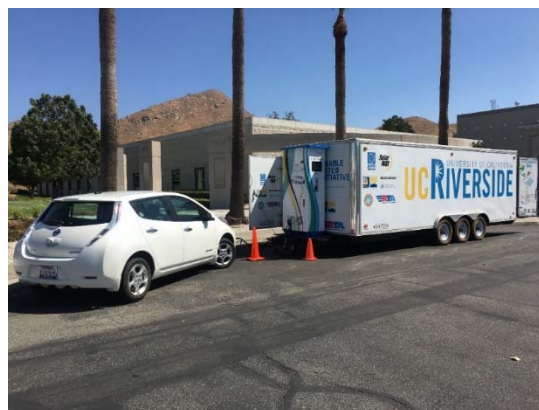
PEV connected to energy storage with V2G capability.
