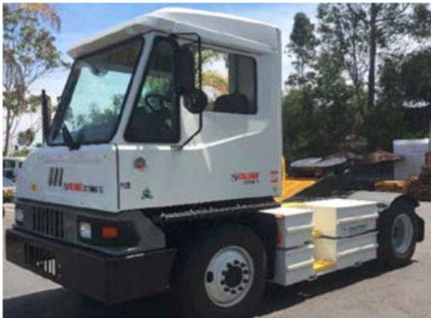
Figure 9: Kalmar/TransPower Battery-Electric Yard Truck
