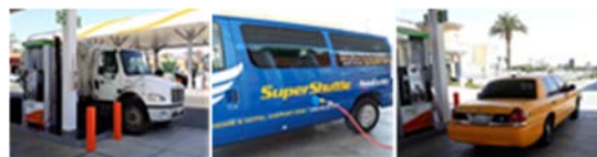
Fig. 4 CNG fueling of Street Sweeper, Airport Shuttle Van, Passenger Class vehicles
