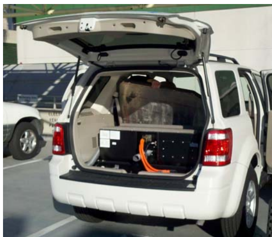
Figure 1: Enerdell battery integrated by Quantum Technologies
