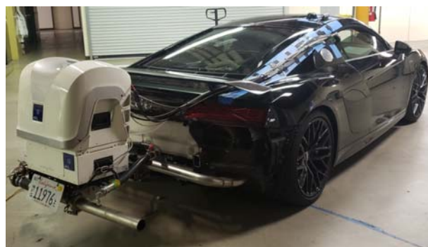
Figure 1: Portable emissions equipment attached to late model automobile.
