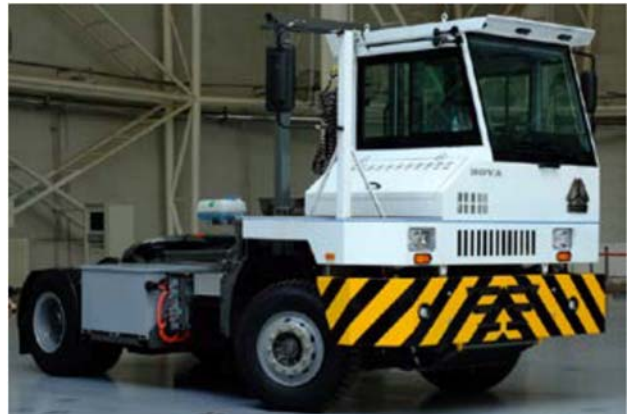
Figure 10: CNHTC/LOOP Energy Fuel Cell Yard Truck
