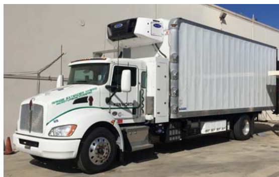
Figure 1: Hybrid Kenworth Class 7 Reefer truck with CNG powered Capstone turbine
