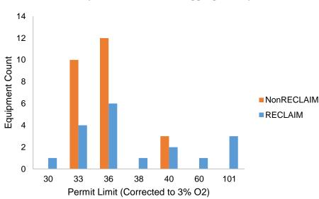
Figure 2-2 – Summary of Assessment on Aggregate Dryer Permit Limits
