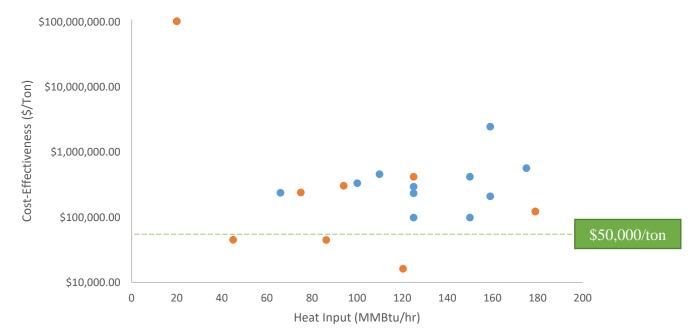
Figure 2-3 – Cost Effectiveness Estimate for Aggregate Dryers
