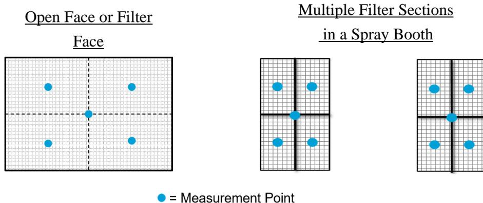
For an enclosed spray booth, the inward face air velocity measurements shall be taken between 6 and 12 inches from the exhaust filters.
