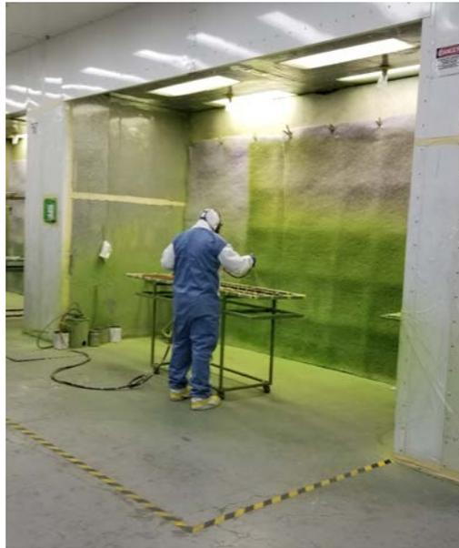
**Figure 2 – Examples of Enclosed Non-Bench Spray Booths**
