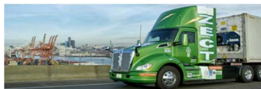
Figure 1: Zero Emission Electric Drayage Truck with Fuel Cell Range Extender
