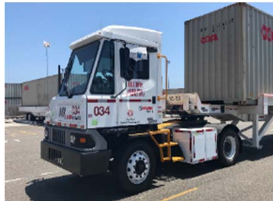
Figure 1. Battery-Electric Kalmar Yard Tractor
