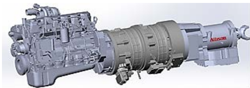
Figure 19: Parallel Hybrid Powertrain: 8.9L ISLG, Dual Electric Motors, Allison Transmission
