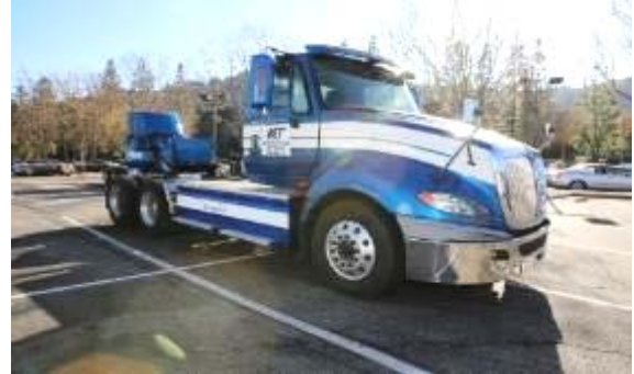
Figure 16: eTruck-2 with 280 kWh NMC 6-Pack
