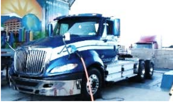
Figure 15: eTruck-1 with 180 kWh LFP 11-Pack
