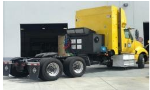
Figure 17 TransPower’s PHET-2 Rear Mounted ICE
