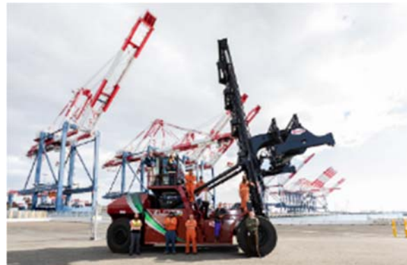
Figure 2. Battery-Electric Taylor Top Handler
