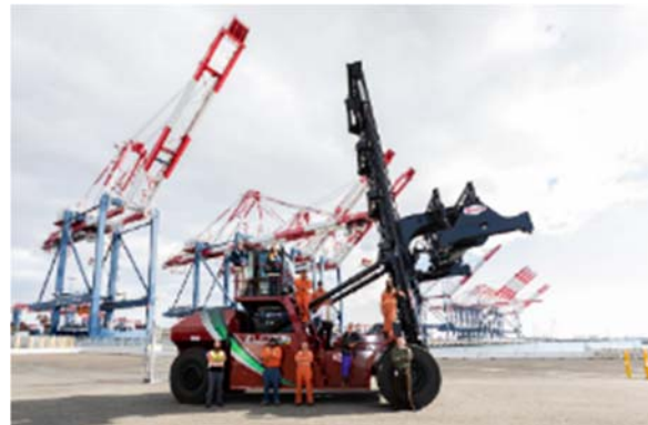
Figure 2. Battery-Electric Taylor Top Handler
