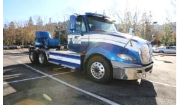
Figure 16: eTruck-2 with 280 kWh NMC 6-Pack
