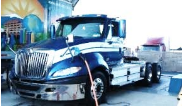
Figure 15: eTruck-1 with 180 kWh LFP 11-Pack
