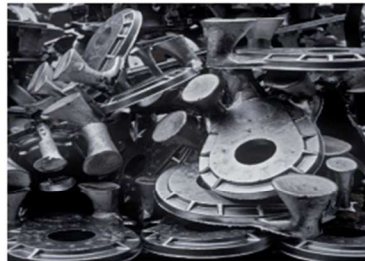
Casting w/ risers (multiple metals)
