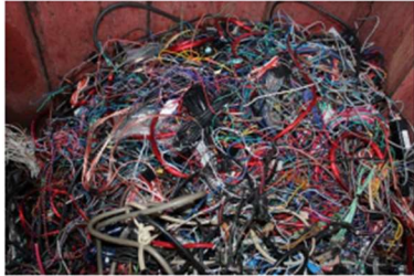
Insulated Scrap Wire (Copper or Aluminum)
