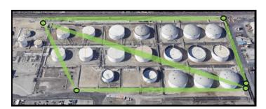
Figure 4.10 – Implementation of Open Path Detection (Example)
