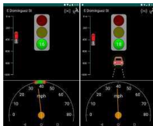
User Interface of Connected Eco-driving Application
