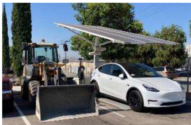
Figure 16: L25 Charging on Solar Charger
