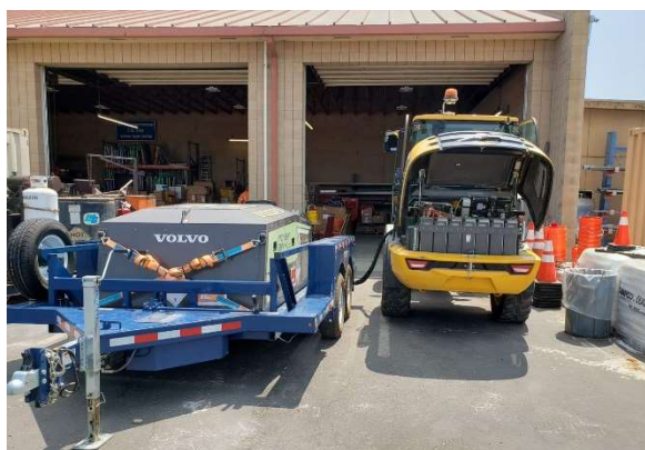
Figure 2 – L25 Being charged by Mobile Battery Bank
