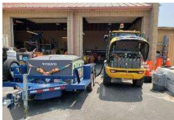
Figure 15: L25 Being Charged by Mobile Battery Bank
