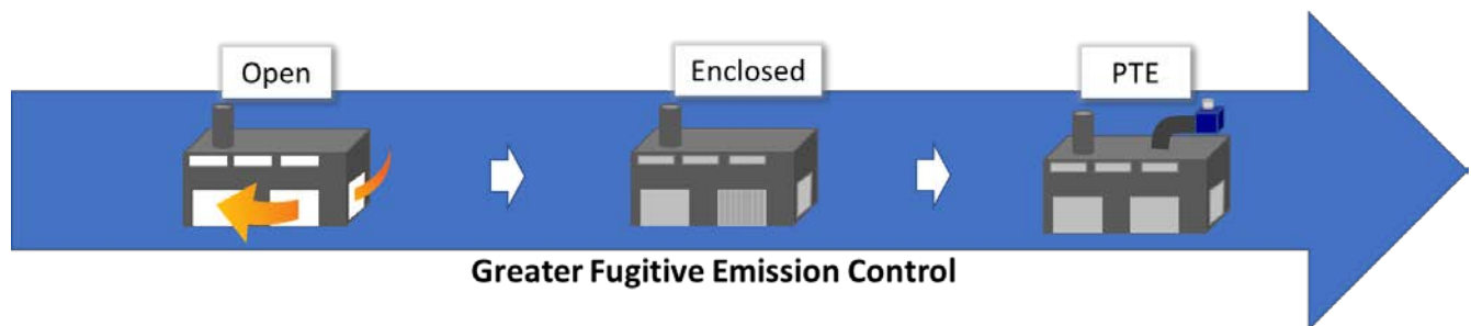
Figure 1-16 – Examples of Building Enclosures to Reduce Fugitive Emissions
