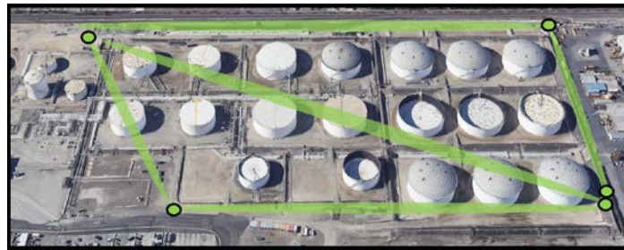
Figure 4.10 – Implementation of Open Path Detection (Example)
