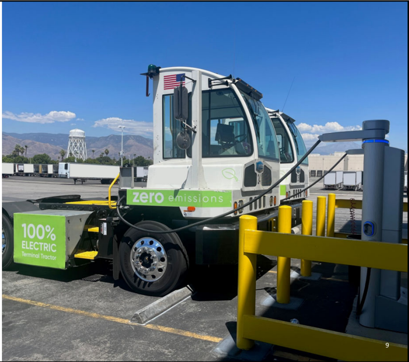
ZE yard truck (hostler) with Level 2 Charger at a warehouse in San Bernardino County
