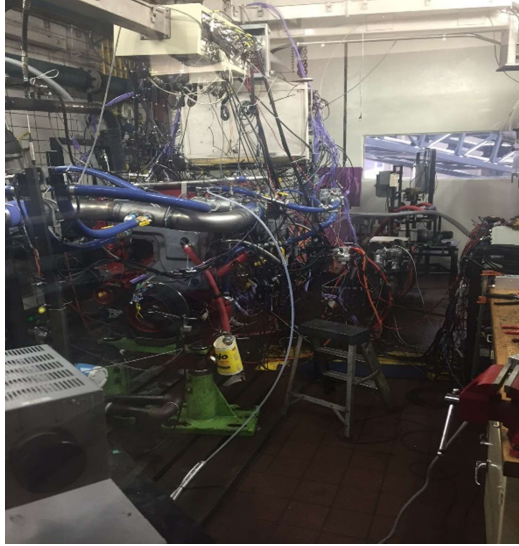
Figure 1: Test Engine on Dynamometer
