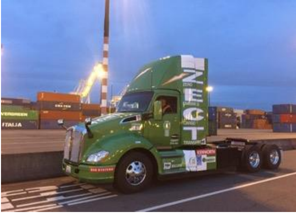
Figure 6: Kenworth Fuel Cell Truck
