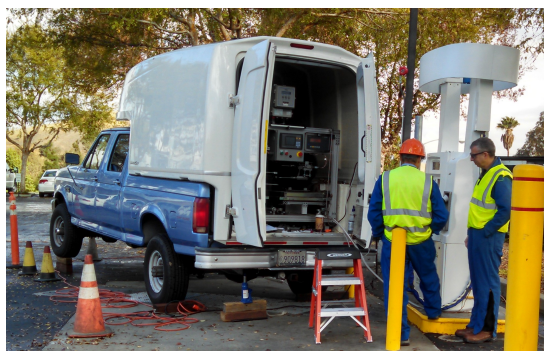
Figure 1: DMS staff testing a hydrogen dispenser
