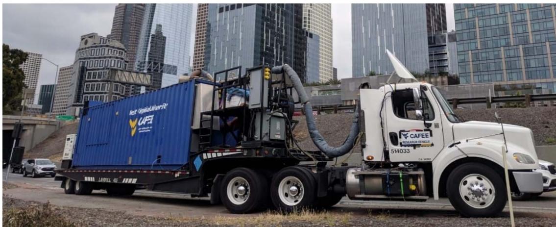
Figure 6: Real-World In-Use Emissions Testing with Lab-Grade Equipment
