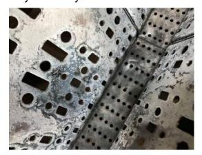
Picture 2 – Close Up of Burner Ports
