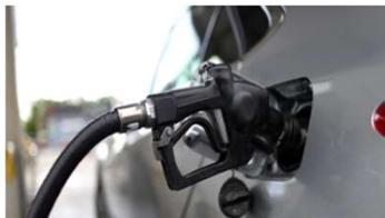
Phase II vapor recovery systems capture vapors during dispensing fuel into motor vehicles
