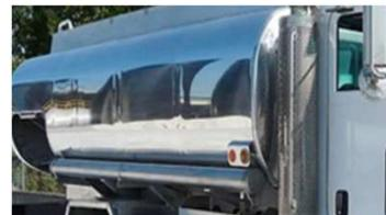
Tank surface color and insulation lowers temperature to reduce evaporative emissions
