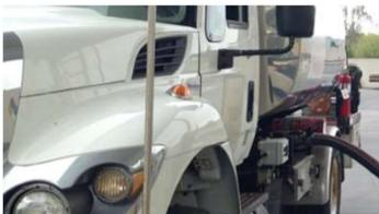
Phase I vapor recovery systems capture vapors during dispensing into tank of mobile fueler
