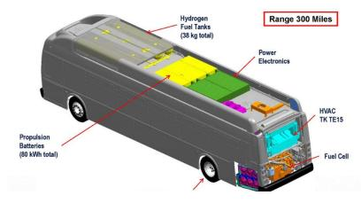
Figure 12: Features of Fuel Cell Transit Bus
