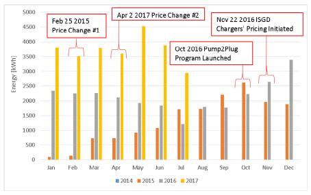
Figure 2: Energy consumption of MSTB charging station during demonstration
