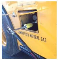
Figure 2: Bus Fueling with Slow-Fill Nozzle
