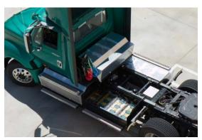
Figure 1: A demonstration vehicle equipped with Inverter-Charger Unit
