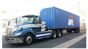
Figure 2: eTruck™ 1 with 80,000 lbs GCWR
