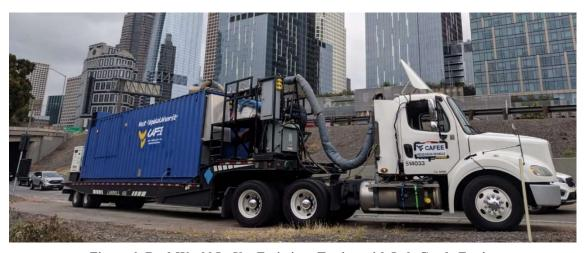
Figure 6: Real-World In-Use Emissions Testing with Lab-Grade Equipment
