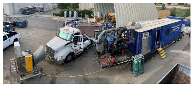
Figure 5: Chassis Dyno Setup for a Goods Movement Truck
