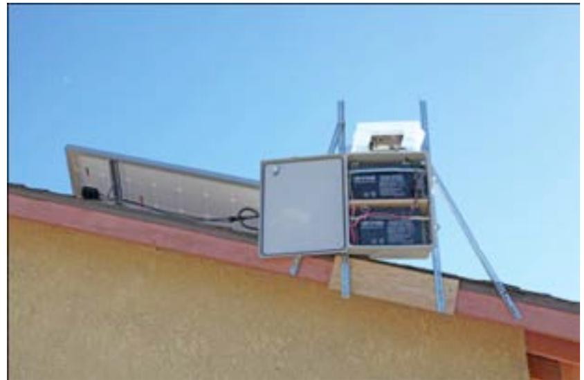
**AirBase Multi-Sensor Air Quality Monitoring Station Version II**
