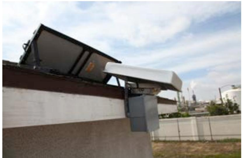
**AirBase Multi-Sensor Air Quality Monitoring Station Version I**
