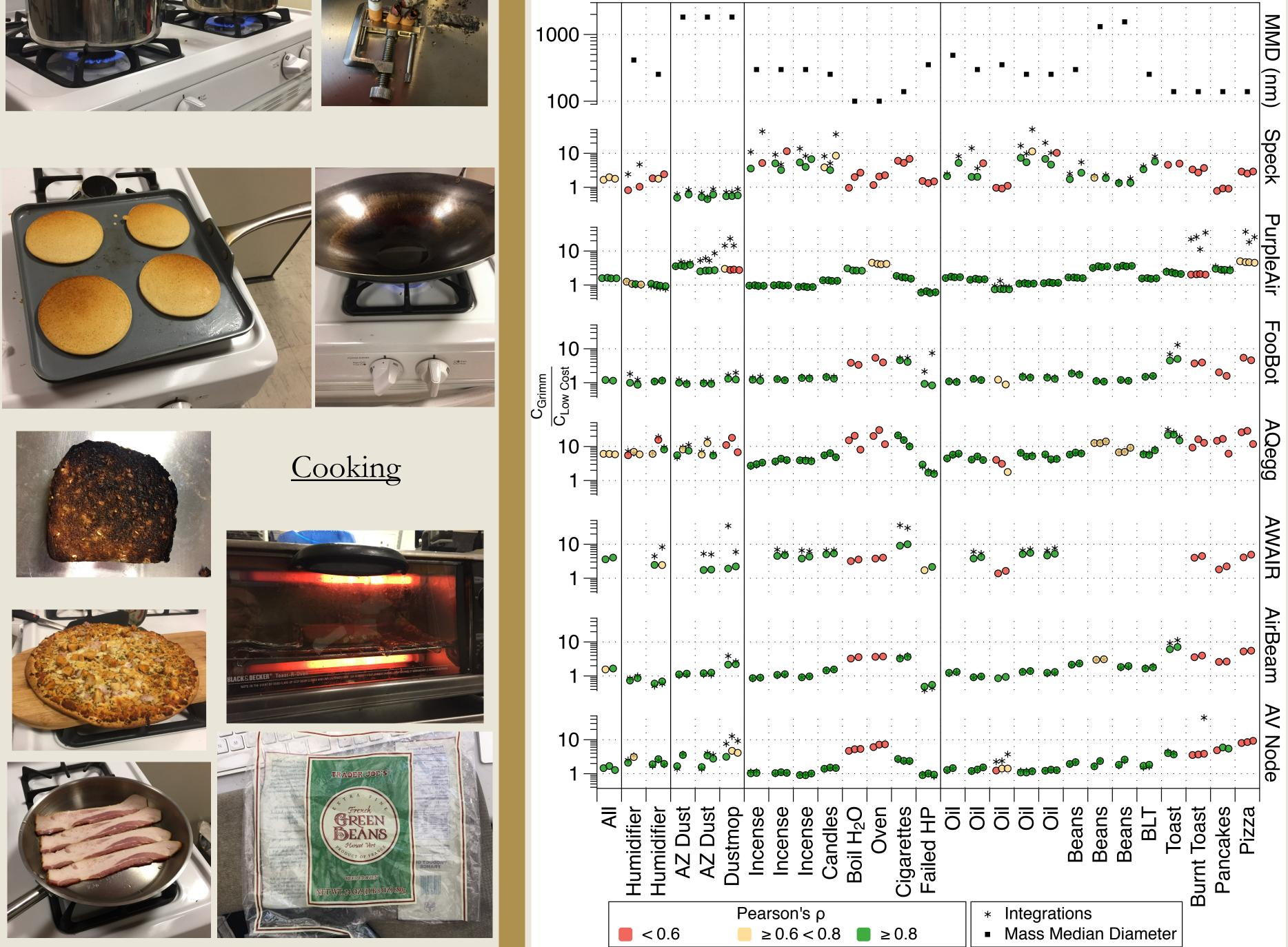
Approach We performed a series of scripted events in a lab space the size of a large residential room. The events covered a range of possible indoor sources. Each test involved a pre-release period, the actual event, a 1-hr decay followed by a room flush. Low cost, reference, and research monitors were centrally placed in the well mixed room.
