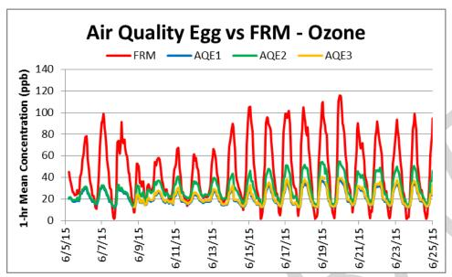
Ozone measurements from all three AQE sensors correlate very well with the corresponding FRM data (0.85<R2<0.87), but they largely underestimate FRM measured Ozone concentrations
