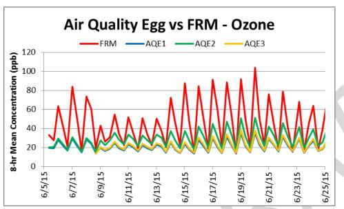
Ozone measurements from all three AQE sensors correlate very well with the corresponding FRM data (0.84<R2<0.87), but they largely underestimate FRM measured Ozone concentrations
