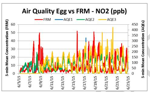
NO2 measurements from all three AQE sensors correlate poorly with the corresponding FRM data (0.34<R2<0.40) and overall, they overestimate measured NO2 concentrations
