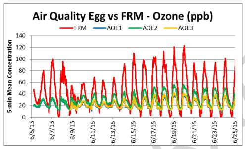
Ozone measurements from all three AQE sensors correlate very well with the corresponding FRM data (0.84<R2<0.86), but they largely underestimate FRM measured Ozone concentrations
