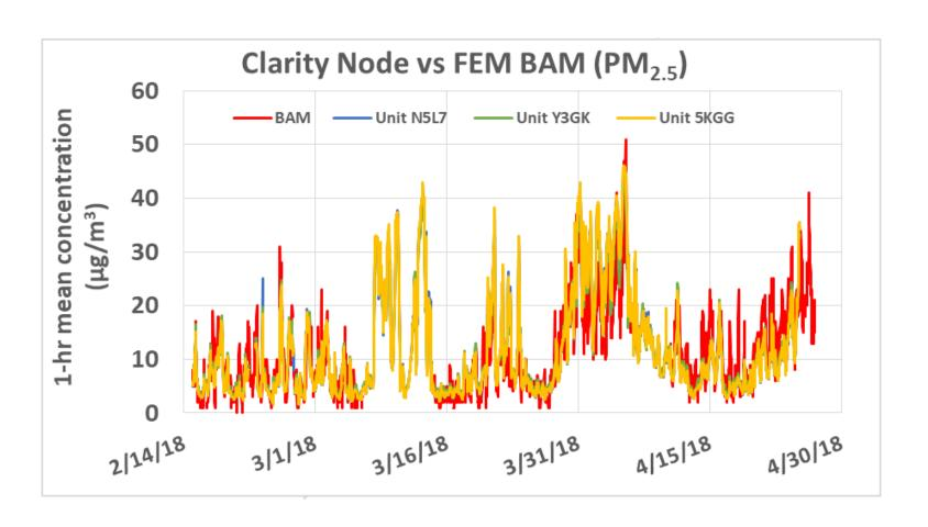
Clarity Node sensors track well the diurnal PM<sub>2.5</sub> variations recorded by the FEM BAM instrument
