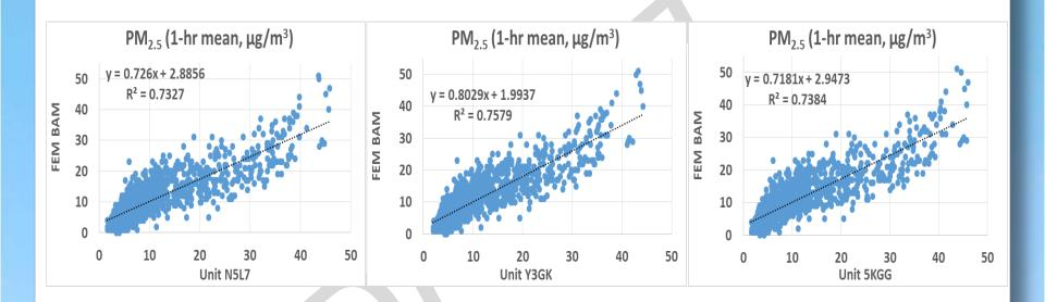
Clarity Node PM<sub>2.5</sub> mass measurements correlate well with the corresponding FEM BAM data (R<sup>2</sup> > 0.73)
