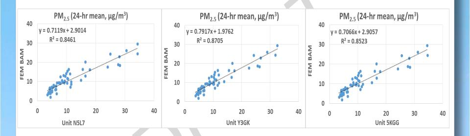
Clarity Node PM<sub>2.5</sub> mass measurements correlate well with the corresponding FEM BAM data (R<sup>2</sup> > 0.84)
