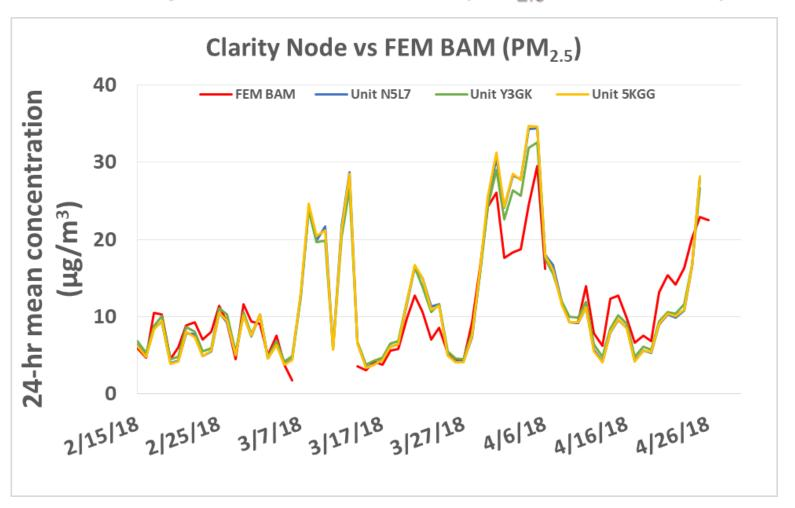
• Clarity Node sensors track well the diurnal PM<sub>2.5</sub> variations recorded by the FEM BAM instrument
