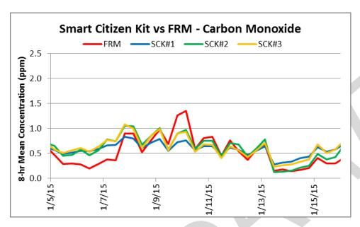
Overall, all CO measurements correlate well with the corresponding FRM data (0.45<R2<0.82)</li>
