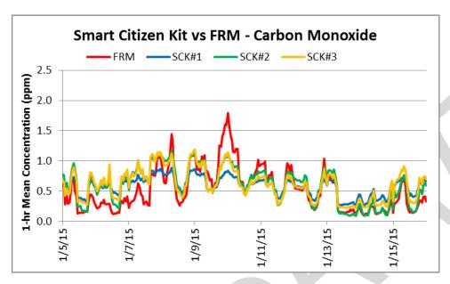
Overall, all CO measurements correlate well with the corresponding FRM data (0.49<R<sup>2</sup><0.84)</li>
