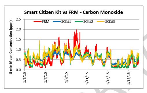
Overall, all CO measurements correlate well with the corresponding FRM data (0.48<R<sup>2</sup><0.83)</li>
