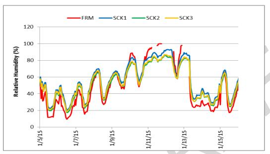
All SCK RH measurements correlate very well with the corresponding reference (station) RH data (R<sup>2</sup>>0.97)
