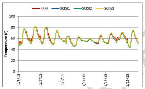
All SCK Temperature measurements correlate very well with the corresponding reference (station) temperature data (R<sup>2</sup>>0.94)
