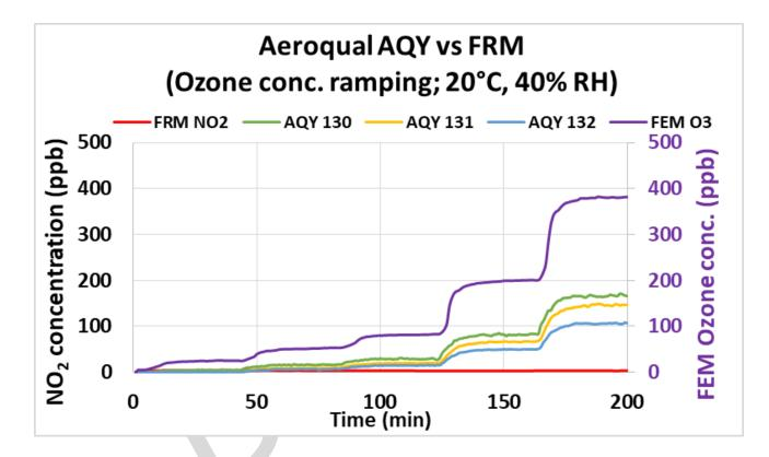
In the laboratory, the effect of  $O_3$  interferent was evaluated by exposing sensors to increasing  $O_3$  concentrations at 20 °C and 40% RH. As shown in the figure, the FRM NO<sub>2</sub> measurements maintained their baseline readings throughout the O<sub>3</sub> concentration ramping from 0 to ~ 400 ppb while the Aeroqual AQY sensors showed increasing NO<sub>2</sub> concentrations as O<sub>3</sub> interferent concentration increased from 0 to ~ 400 ppb.
