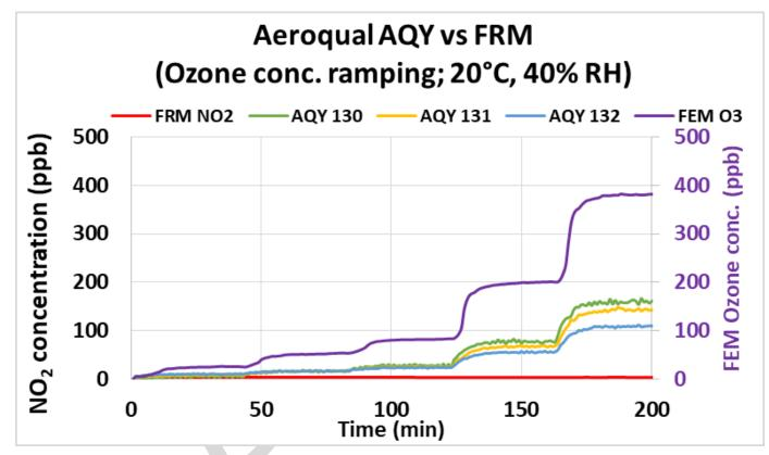
In the laboratory, the effect of  $O_3$  interferent was evaluated by exposing sensors to increasing concentrations of  $O_3$  at 20 °C and 40% RH. As shown in the figure, the FRM NO<sub>2</sub> maintained their baseline readings throughout the  $O_3$  concentration ramping from 0 to ~ 400 ppb while the Aeroqual AQY sensors showed increasing NO<sub>2</sub> concentrations as  $O_3$  interferent concentration increased from 0 to ~ 400 ppb.
