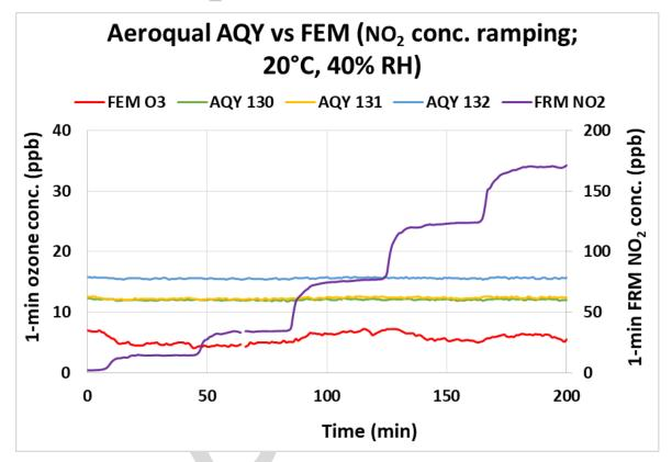
In the laboratory, the effect of NO<sub>2</sub> interferent was evaluated by exposing sensors to increasing concentrations of NO<sub>2</sub> at 20 °C and 40% RH. As shown in the figure, both the FEM and Aeroqual AQY O<sub>3</sub> measurements were not affected by the NO<sub>2</sub> interferent and maintained their baseline readings throughout the NO<sub>2</sub> concentration ramping from 0 to ~ 150 ppb.
