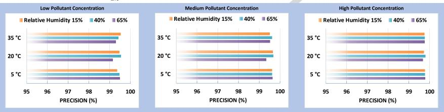
Overall, the two Clarity Node sensors showed high precision for all of the combinations of low, medium and high PM<sub>2.5</sub> conc., T, and RH.
