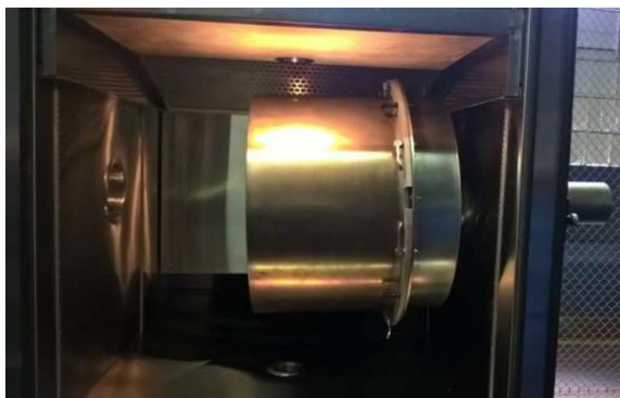
Figure 5. Inner chamber installed inside the outer chamber; This configuration is exclusively used for testing gaseous sensors
