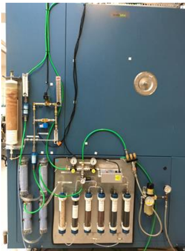
Figure 2. Dry, gas- and particle-free air system (or zero-air system)
