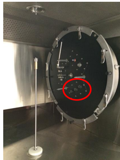
Figure 9a-b. Sensor communication (USB) and power ports “plate” (a) and communication “plate” installed on inner chamber base (b)
