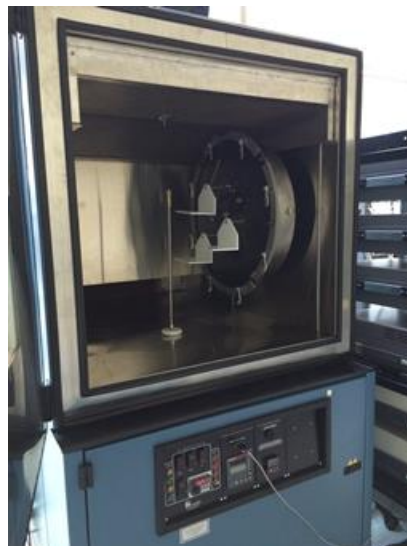
Figure 3. Inside view of the outer chamber; PM sensors are placed on three Teflon trays (in white) for testing
