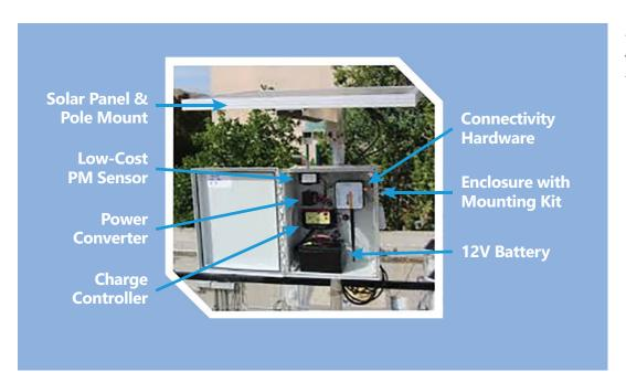
**Figure 3-10.** An example of a sensor system.
