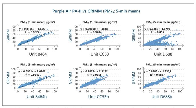
**Figure 3-9.** Excerpt of an AQ-SPEC field evaluation of the PurpleAir PA-II. See Chapter 4 for discussion of scatter plots and linear regression.
