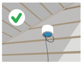
**Good location:** The sensor has good air flow and is sheltered from the elements.
