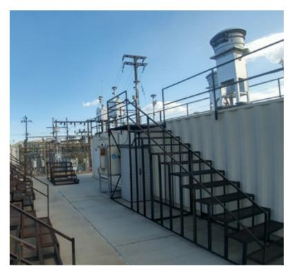
Figure 2-3. Example of a regulatory ambient monitoring station (South Coast AQMD Riverside-Rubidoux site).
