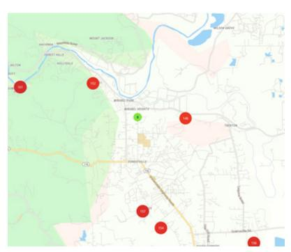
*Figure 4-16.* PurpleAir map of concentrations observed during a wildfire smoke event in Northern California. The sensor with low concentrations (green dot) is suspect given the widespread smoke conditions.
