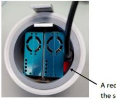
A red LED will be on when the sensor is powered.
