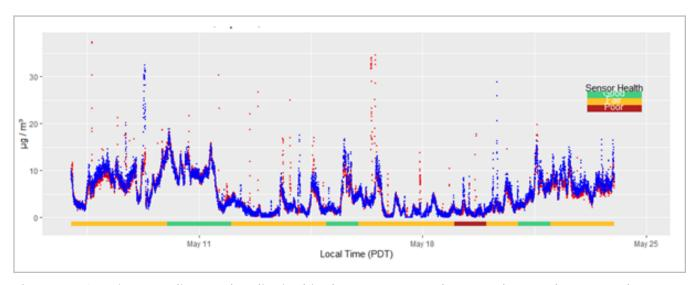
Figure 4-7. Sample plot created using the function 'pat\_dailySoHIndexPlot()' in the AirSensor package.
