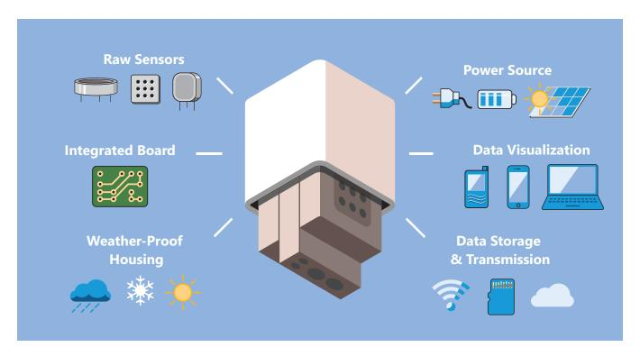
**Figure 2-5.** Basic components of a sensor system.
