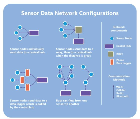
Figure 3-11. Various sensor data network configurations.
