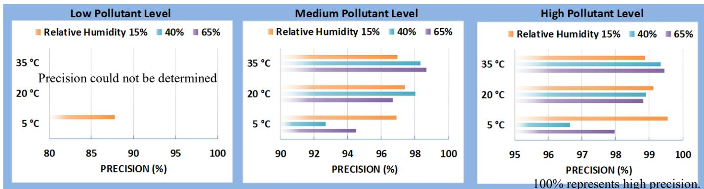
Sensor's ability of generating precise measurements of NO<sub>2</sub> concentration at low, medium, and high pollutant levels were evaluated under 9 combinations of T and RH, including extreme weather conditions like cold and dry (5 °C and 15%), cold and humid (5 °C and 65%), hot and humid (35 °C and 65%), or hot and dry (35 °C and 15%).
