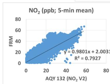
Coefficient of Determination ( $R^2$ ) quantifies how the two sensors (units 130 and 132) followed the NO<sub>2</sub> concentration change measured by the FRM instrument.
