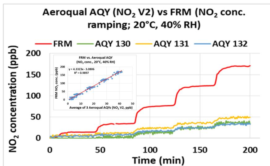
The three Aeroqual AQY sensors showed very strong correlations with the corresponding FRM data ( $R^2 \sim 0.99$ ) at 20 °C and 40% RH.
