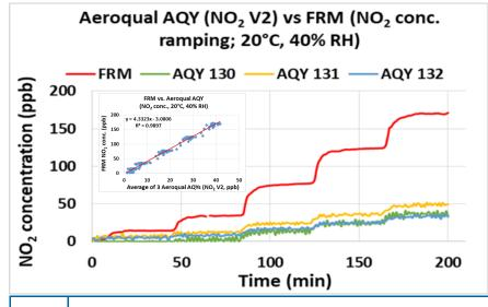
The three Aeroqual AQY sensors showed very strong correlations with the corresponding FRM data ( $R^2 \sim 0.99$ ) at 20 °C and 40% RH.
