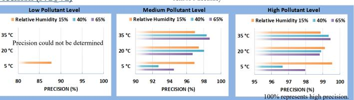
Sensor's ability of generating precise measurements of NO<sub>2</sub> concentration at low, medium, and high pollutant levels were evaluated under 9 combinations of T and RH, including extreme weather conditions like cold and dry (5 °C and 15%), cold and humid (5 °C and 65%), hot and humid (35 °C and 65%), or hot and dry (35 °C and 15%).
