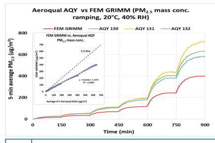
The three Aeroqual AQY sensors showed excellent correlation with the corresponding FEM  $PM_{2.5}$  data ( $R^2 > 0.99$ ) at 20 °C and 40% RH.
