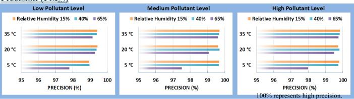
Sensor's ability of generating precise measurements of PM concentration at low, medium, and high pollutant levels were evaluated under 9 combinations of T and RH, including extreme weather conditions like cold and dry (5 °C and 15%), cold and humid (5 °C and 65%), hot and humid (35 °C and 65%), or hot and dry (35 °C and 15%).
