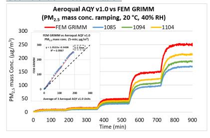
The Aeroqual AQY v1.0 sensors showed very strong correlations with the corresponding FEM PM<sub>2.5</sub> data ( $R^2 > 0.99$ ) at 20 °C/40% RH.
